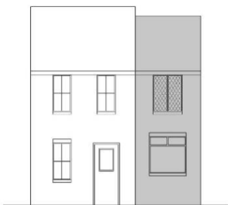
Inappropriate window proportion and style
