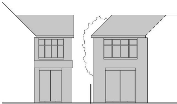
Insufficient gap between properties and roof forms incompatible
