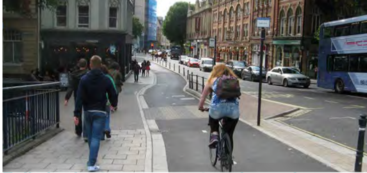
Fully kerbed segregated cycle track
