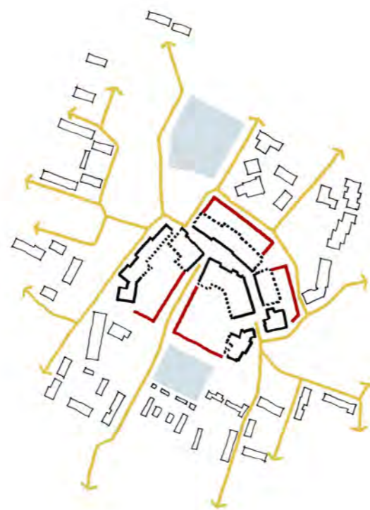
Sketch of New Ash Green shopping centre showing the principle of working with and completing the existing urban form
