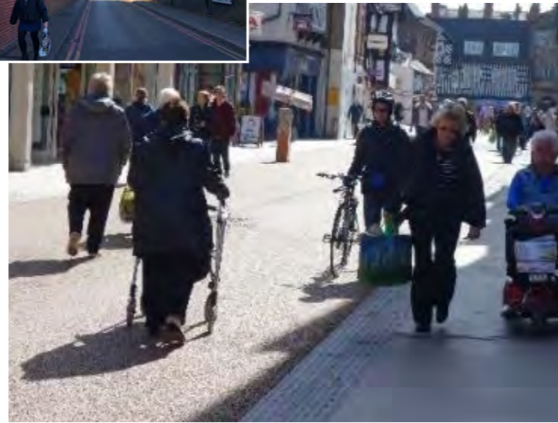
Frodham Street Chester. Example of a pedestrian priority street, level street surface. As part of upgrades the street was decluttered to provide unobstructed pedestrian movement. The scheme uses relatively low cost contrasting surfacing, which could also be applied to Swanley's car parking areas and pedestrian routes such as Nightingale Way (pictured above) ©photo by David Mckenna, Frodham Street, Chester designed by Mott MacDonald and IBI Group
