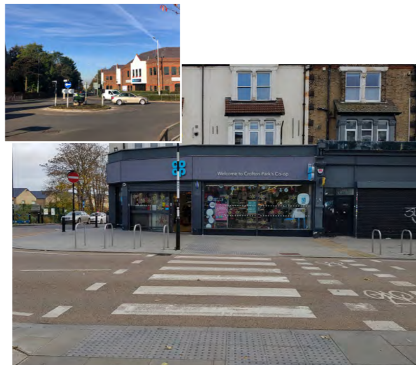
An example of a raised table pedestrian and cyclist crossing with contrasting surfacing. In Swanley, controlled crossings in place of roundabouts would help to improve pedestrian and cyclist accessibility into the town centre.
